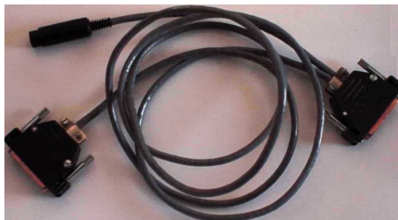
Figure 2: A parallel cable to genlock 2 machines. Beside the two DB25 connectors, we can distinguish a female mini-din 3 connector to plug the IR emitter of the shutter glasses.
