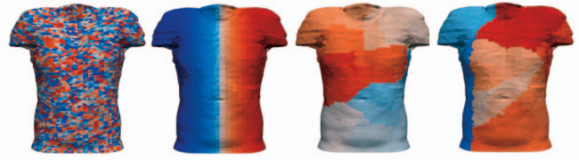
Fig. 3. Visual illustration of different layouts for the torso mesh. Successive cells in memory are colored from blue to red. From left to right, the original, geometric (sorted by x , y , and z -coordinates), OpenCCL (cache-coherent layout from [5]) and FastCOL (our approach) layouts. For spatially close tetrahedra, color discrepancy decreases from the left to right layouts. It denotes an improved memory locality, less likely to generate cache-misses for spatially coherent access patterns.
