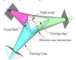
Figure 2: Visual hull of a sphere with 3 views.
