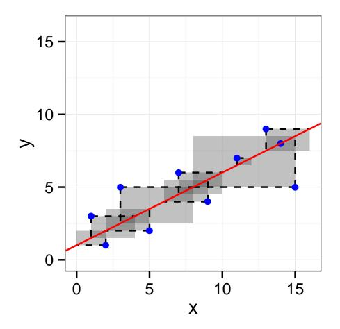
Minimize E(α, β) = ∑<sub>i=1</sub><sup>n</sup> |x<sub>i</sub> - y<sub>i</sub> - α | ⋅ |y<sub>i</sub> - α - βx<sub>i</sub>|
