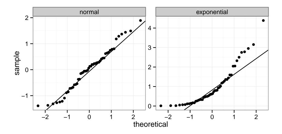
A quantile-quantile plot is a graphical method for comparing two probability distributions by plotting their quantiles against each other
