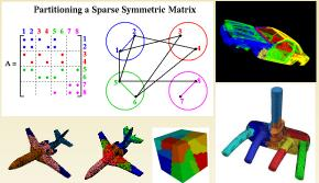
When using adaptive mesh-refining, load imbalance occurs. Coupling code makes it worse.
