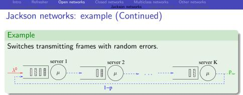
Using M/M/1 results for each queue we get the mean number of frames at each queue  $\mathbb{E}[X_i] = \frac{\lambda^0}{p\mu - \lambda^0}$ The expected transmission time of a frame is therefore (Little)
