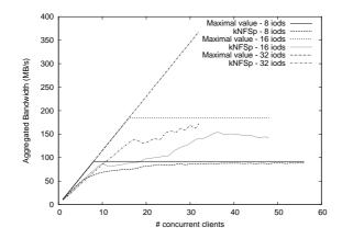
Fig. 5. Comparison user-mode server - kernel-mode NFSP server - with a varying number of iods  $% \mathcal{F}(\mathcal{F})$
