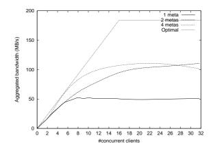
Fig. 3. Aggregated bandwidth with a varying number of meta-servers and clients - 16 iods
