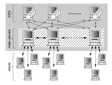
Fig. 1. Distributed metaserver architecture of dNFSp
